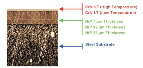
Figure 1: Cross section of the sample showing the different layers CrN, NiP and Steel substrate
