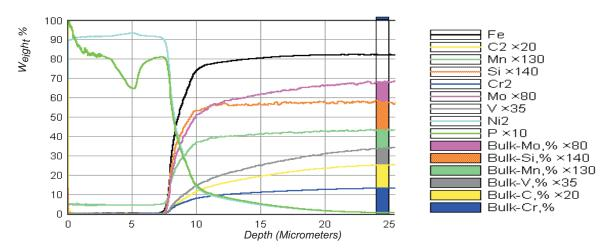
Figure 16: Bulk analysis of the substrate made from the Depth Profile Analysis
